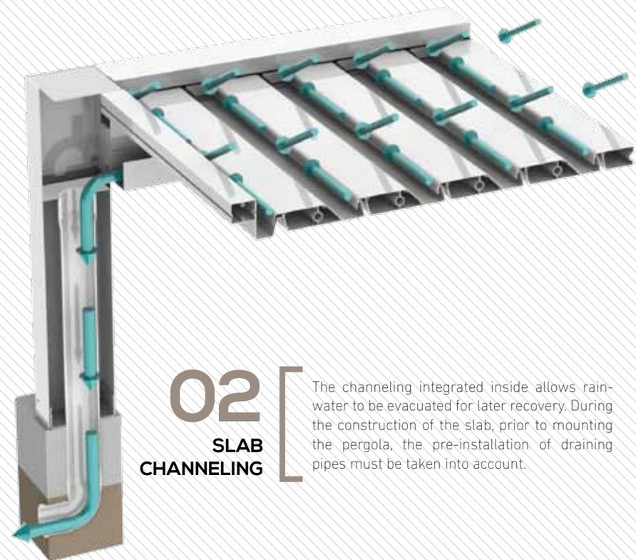
The channeling integrated inside allows rainwater to be evacuated for later recovery. During the construction of the slab, prior to mounting the pergola, the pre-installation of draining pipes must be taken into account.
