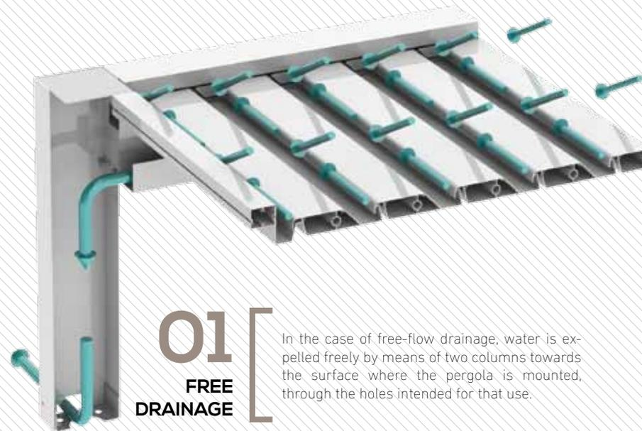
In the case of free-flow drainage, water is expelled freely by means of two columns towards the surface where the pergola is mounted, through the holes intended for that use.
